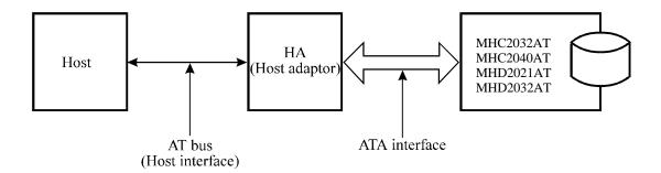
Figure 2.3 1 drive system configuration
